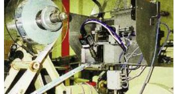
Air heater and blower for drying labels. Fast drying allows for high throughput speeds.
